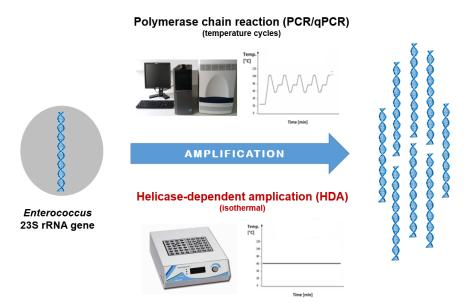
Figure 1: Schematic representation of instrument complexity and temperature requirements for polymerase chain reaction (PCR) and helicase-dependent amplification (HDA) technology
