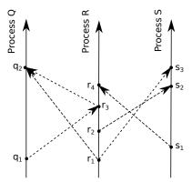
**Figure 1:** An example of parallel processing modeled as partial order; arrows denote the order/precedence relation
