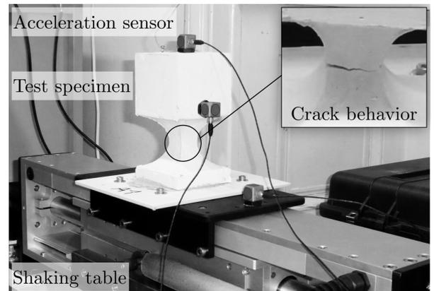
**Figure 2:** Setup for the limit state test
