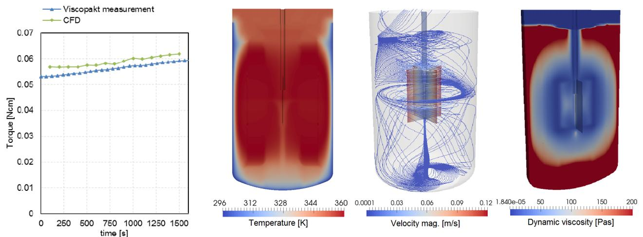
Figure 1 Comparison of the calculated and measured value of the torque (left), selected contour plots<sup>[6]</sup> of the CFD simulation at  $t = 1500$  s (right)
